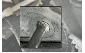
Image 1: The stud is not correctly screwed in
